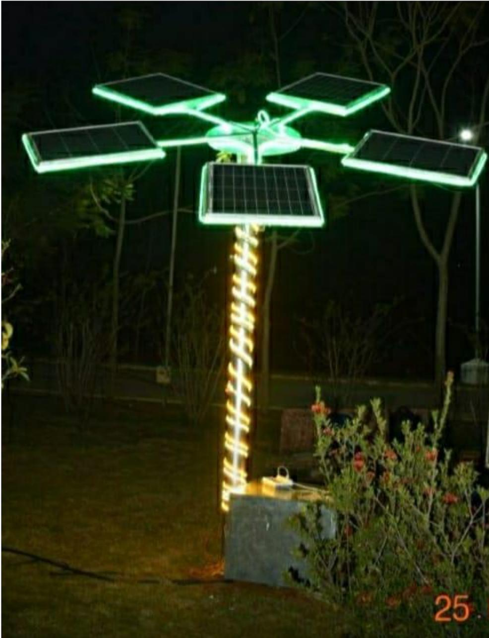
Fig.2. Developed solar tree for EV charging
