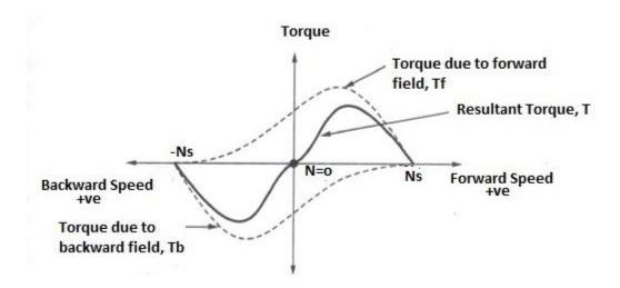
Fig: 1.51(g) Torque-Speed characteristics
